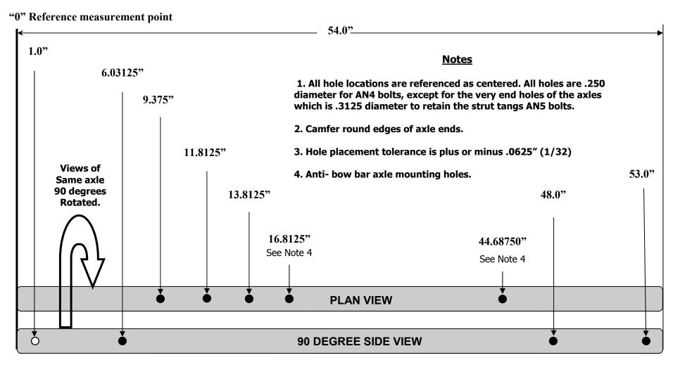
Axle has a finished overall length of 54." It is a length of 6061T6 Aluminum 1.0" O.D. solid bar round stock and weighs 4.0 lbs when finished to install. Not recommended for aircraft whose pilots weigh more than 170 lbs., because it will bend. Use a steel axle for heavier pilots.
