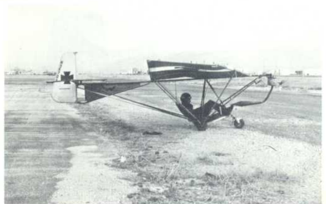
Pilot Sits At C.G., Surrounding Structure Provides Some Protection
