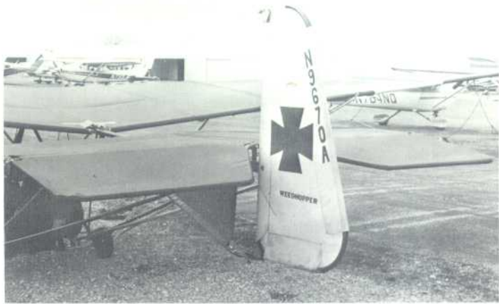
Side Mounted Control Stick Operates Large And Effective Rudder And Elevators.
