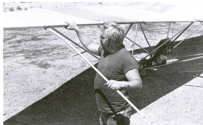
6. Slip ribs in place.
