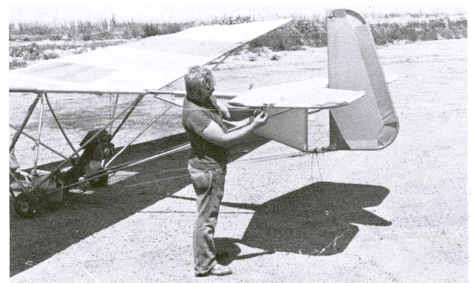
7. Attach elevator brace wires.
